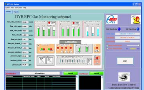
RPC GAS Monitoring GUI
