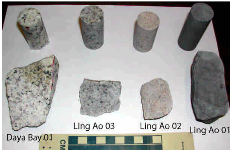
Figure 2. Hand specimens and 1-inch core plugs from the Daya Bay and Ling Ao quarries
