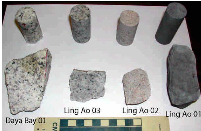
Figure 2. Hand specimens and 1-inch core plugs from the Daya Bay and Ling Ao quarries
