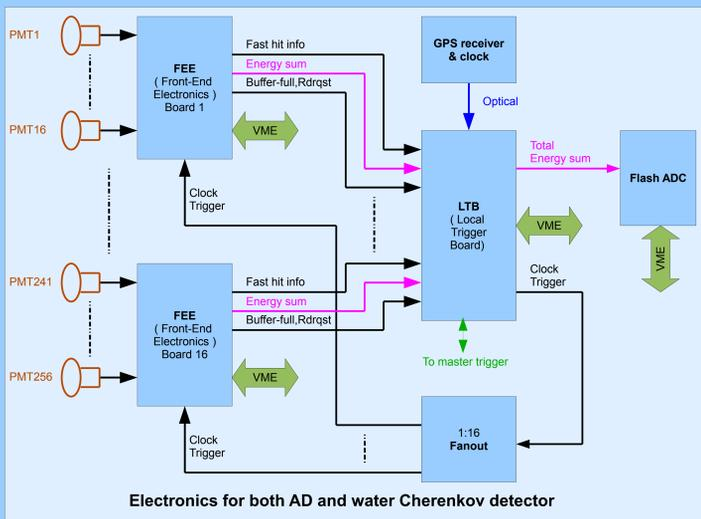
Since both AD and water Cherenkov detector are PMT based, an identical readout electronics subsystem is developed.
