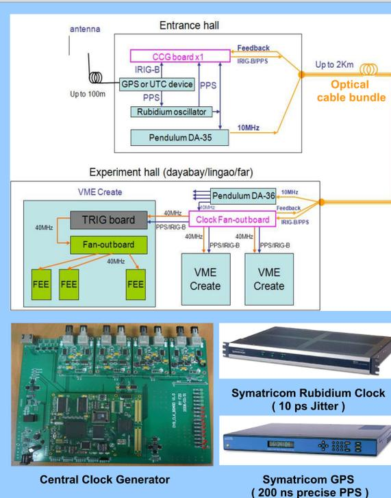
A 10 MHz clock and the absolute time base on a Central Clock Generator (CCG) are generated in the control room outside of the tunnel
