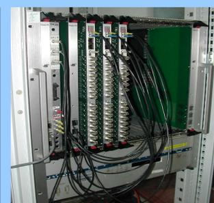
FEE PCB: 8 layer VME module      3 prototype FEE modules under testing
