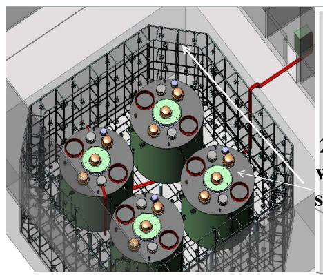
Muon tagging Shielding of background radiation RPC as muon veto on top of water Cherenkov
