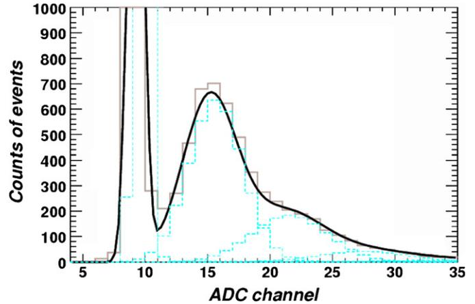
Fig. 3. Fitted spectrum for PMT gain calibration.
