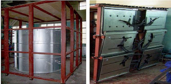
Fig. 2. The prototype detector: rack to mount the muon veto (left) and the mounted muon veto detectors (right).
