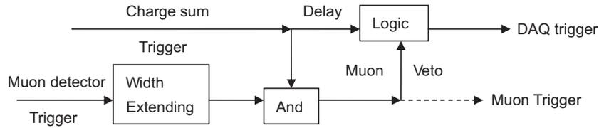
Fig. 4. Block diagram of DAQ.
