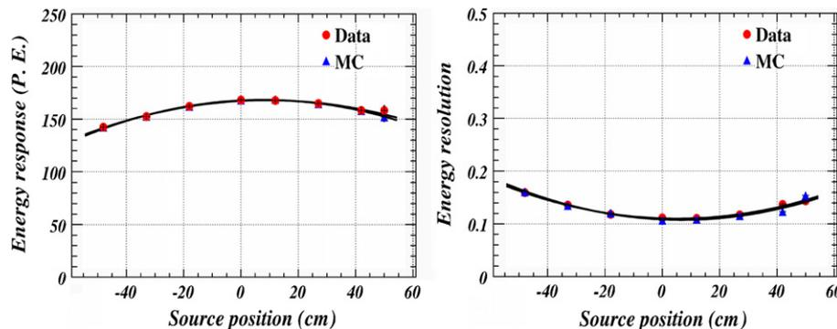
Fig. 9. Energy response of  $^{137}\text{Cs}$  at different locations along the cylindrical central axis in comparison with Monte Carlo simulation.
