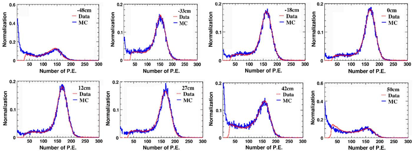
Fig. 8. The spectra of  $^{137}\text{Cs}$  at different locations along the cylindrical central axis, and the comparison with Monte Carlo simulation.
