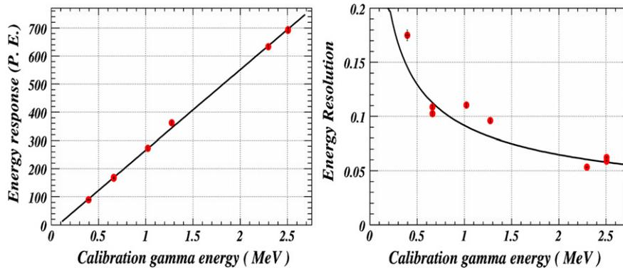
Fig. 7. Linearity of the energy response (left, a) and energy resolution (right, b) of the prototype at the center of the prototype.
