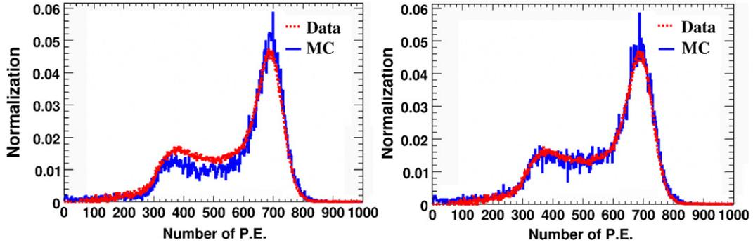
Fig. 5. Energy spectrum of the  $^{60}\text{Co}$  source in comparison with Monte Carlo simulation. Left: no sealing material is included in the simulation. Right: the sealing material is included in the simulation.
