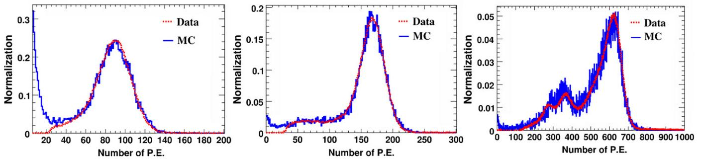
Fig. 6. Comparisons of data and MC spectra of  $^{133}\text{Ba}$  (left),  $^{137}\text{Cs}$  (middle) and  $^{22}\text{Na}$  (right).
