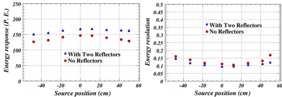
**Fig. 10.** Energy response of the prototype with and without two reflectors for a  $^{137}\text{Cs}$  source at different locations along the central cylindrical axis (energy response (left); energy resolution (left)).
