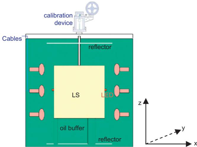
Fig. 1. Side view of the schematic structure of the prototype.
