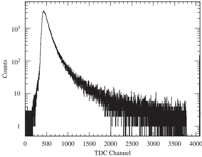
Fig. 2. Decay spectrum of the experimental liquid scintillator, GdLS (after background subtraction [4]).
