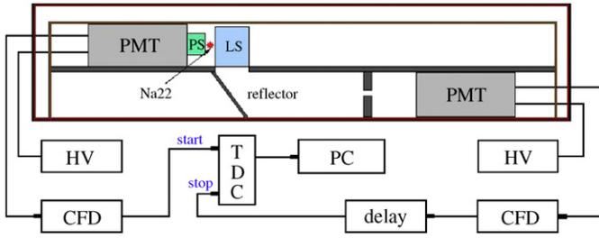
Fig. 1. System setup for the measurement of decay time of liquid scintillator.
