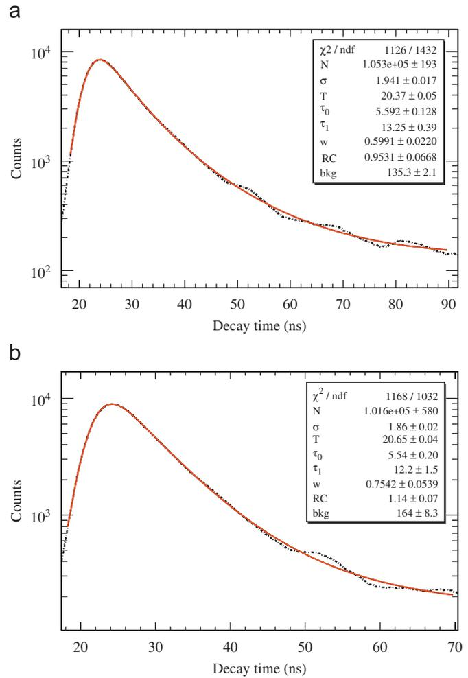
Fig. 5. Pulse shapes of scintillation light recorded by digital oscilloscope and fitting results of parameters. Panel (a) is the result of GdLS and panel (b) is the result of LS.
