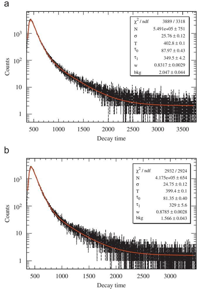
Fig. 3. Fitting results of the two samples of experimental liquid scintillators. (Units of X-axis and the time parameters  $\tau_0$ ,  $\tau_1$ , T,  $\sigma$  are TDC channel.) Panel (a) is the result of GdLS and panel (b) is the result of LS.
