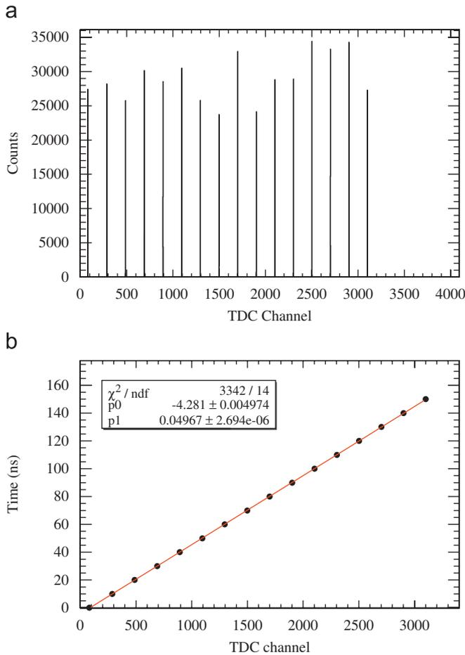
Fig. 4. (a) Calibration spectrum for TDC C414 (200 ns range, 4096 channel) by ORTEC 462 (160 ns range, 10 ns period). (b) Linear fitting results.
